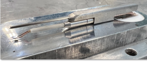
Figure 1: A low-profile sting holding the NSTAP and pitot probe.
